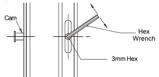
This adjustment can help if the sash is away from the stops or if the lock is difficult to operate.
