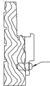
To adjust the catch for the wood screen insert a small wire or allen wrench into the small hole and rotate the plunger to increase or decrease the tension on the screen.
